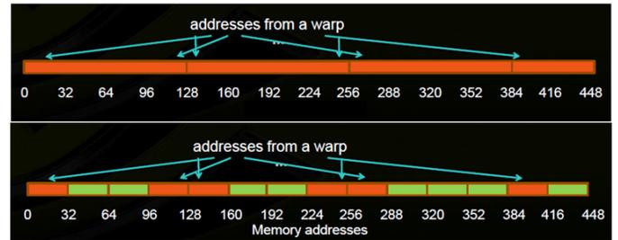
Fig. 7. Fermi offers two modes of scattered global memory access. The top example shows L1 and L2 cache with 128 byte granularity whilst the bottom example shows L2 cache only with 32 byte granularity. The bottom figure represents a more efficient bus utilisation for this implementation.
