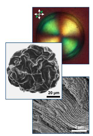
Figure 2: CNCs self-assemble inside aqueous droplets (top) to form cellulose microparticles (middle) with an internal nanostructure order (bottom).
