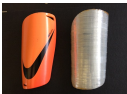
Fig. Football shin pad of Nike Mercurial (left) and the one made of all-PLA composite (right)
